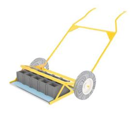
**PRODUCT CARRYING TROLLEY:** it enables the products printed on the pallet from the machine to be transported to the drying area. It is designed according to the size of the production pallets. It is designed for a person to carry the product in the easiest and most convenient way. Large inches for fast movement, pneumatic tires are preferred for comfortable movement on all types of ground. The chassis is made of 34 pipes. The pallet carrying chamber is 4mm sheet metal.
