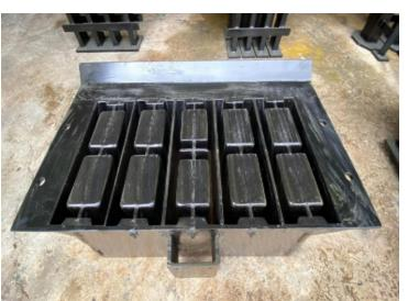
MACHINE MOULD:We process the moulds drawn by using advanced technology on ST 42 / German technology steels in the norm of religion in CNC LASER computerized numerically controlled machines, without touching the hand, with zero error. After induction hardening processes and sensitive carburizing, we obtain anti-wear cobblestone (keystone), block stone, pumice stone, plug-in pumice stone, styrofoam block stone, curb stone, rain gutter, hollow block and chimney stone moulds.
